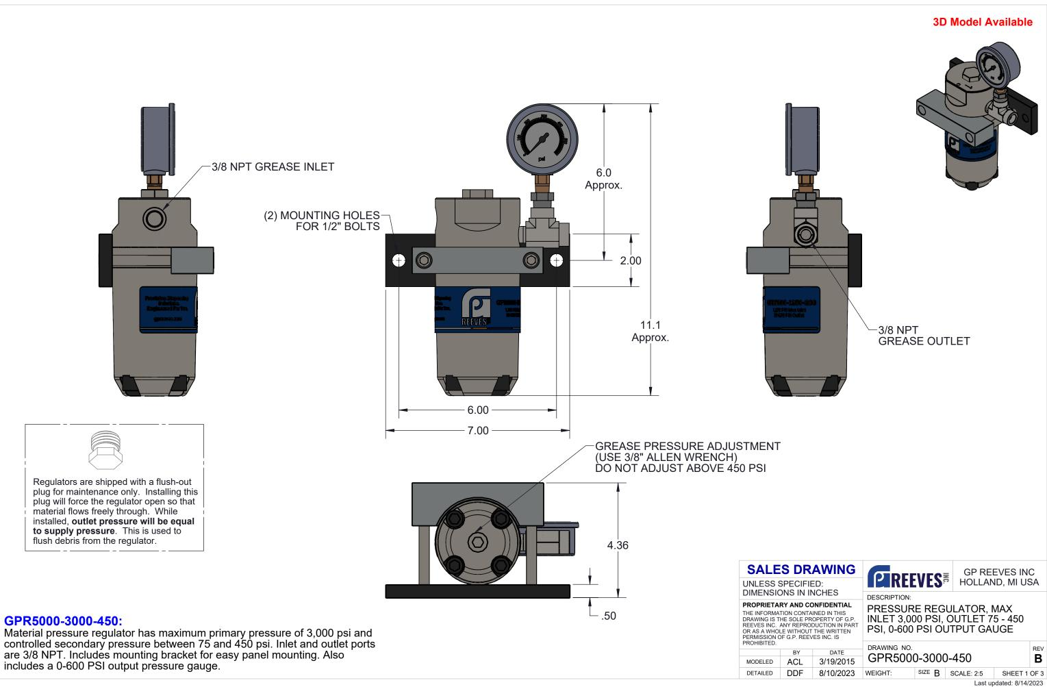
are 3/8 NPT. Includes mounting bracket for easy panel mounting. Also includes a 0-600 PSI output pressure gauge.
